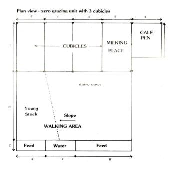
Figure 2.1 Plan view - zero grazing unit with 3 cubicles
