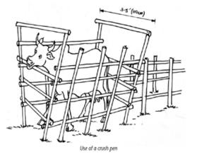
Figure 5.1 Illustration of a crush pen
