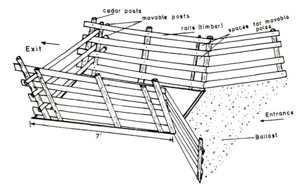
Figure 5.4 Vertical structural design of a crush pen
