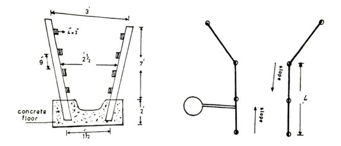
Figure 5.2 Side elevation of a crush pen
