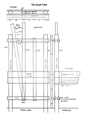
Figure 2.4 View of a head Yoke
